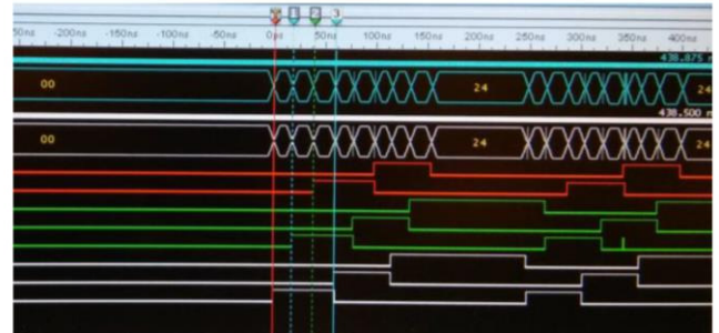
Fig. 4 Verification of external interleaved mode using logic analyzer
