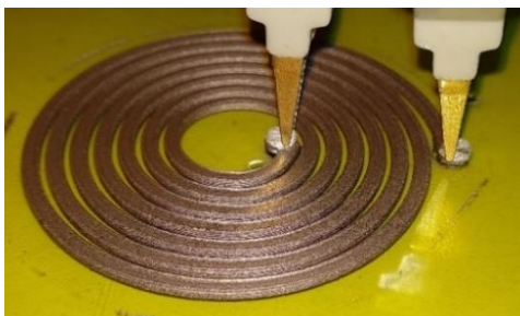
Fig. 4 Measuring inductance of spiral coil using by LCR bridge
