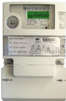
Fig. 5. Three-phase static (digital) meter [7]
