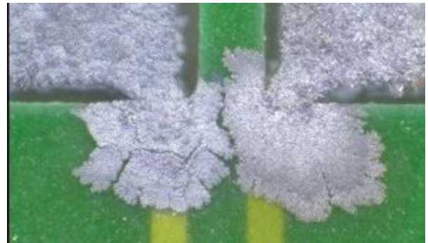
Fig. 3 Detail of Creep corrosion effect of silver coating [9].
