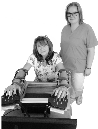
Fig. 1. Device Rehapiano, which includes 10 strain gauges and a keyboard. A monitor is included, but not shown.
