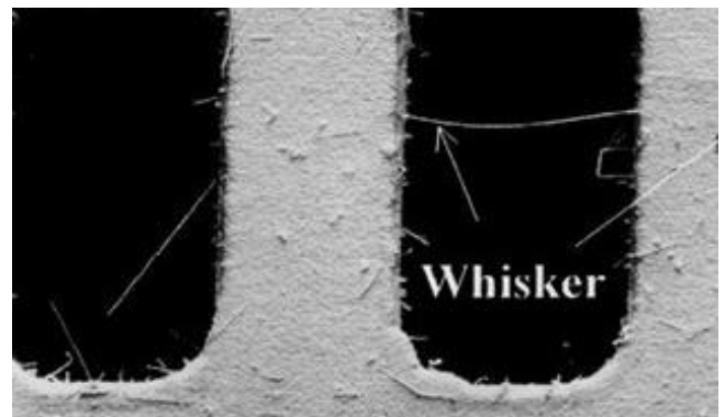
Fig. 4 Detailed view of tin whisker [12].
