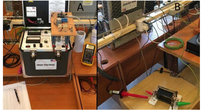
Fig. 2 The experimental setup employed in the breakdown voltage measurements. (A) – High voltage power supply with the output voltage rise rate control system. (B) – BDV test vessel filled with the ferrofluid.
