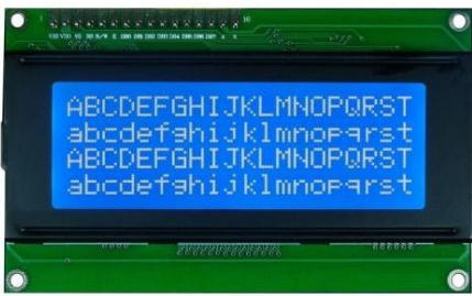
Fig. 5 LCD display QC2004A with HD44780 controller [6]
