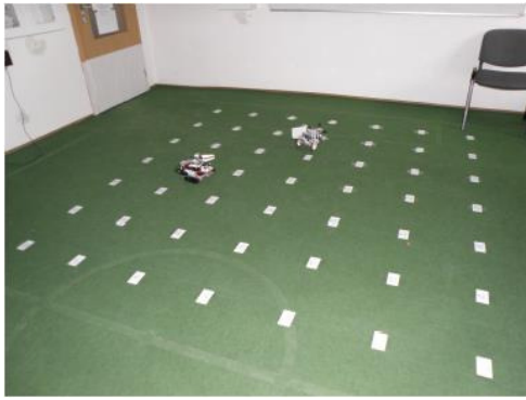
Fig. 3. Testing area with robots and RFID tag grid [5]
