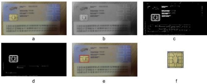
Fig. 2. Input image (a), grayscale (b), edge detection (c), blobs filter (d), selection of region of interest (e), extracted microchips pattern (f).
