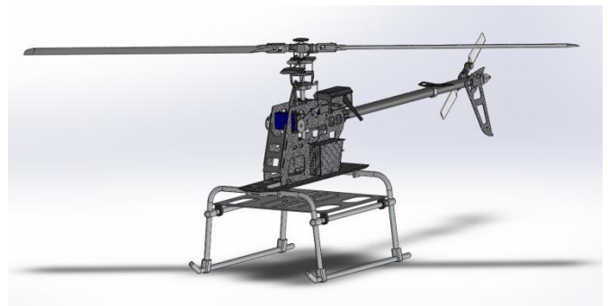
Fig. 6 T-Rex 600 - 3D model for application in Gazebo environment
