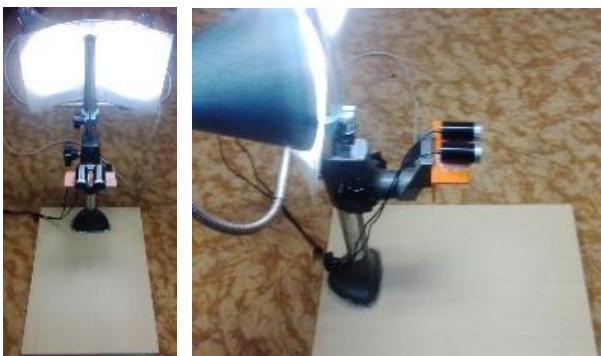
Fig. 2 Assembled parallel stereoscopic system.
