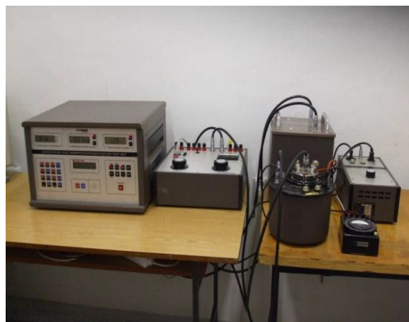
Fig.4 Measurement workplace on measuring C_x and \tan \delta [2].
