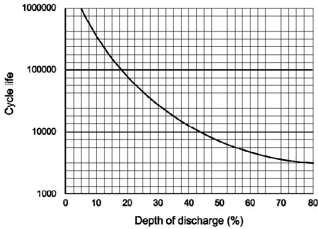
Fig. 3 Cycle-life curve for the Saft lithium-ion battery system
