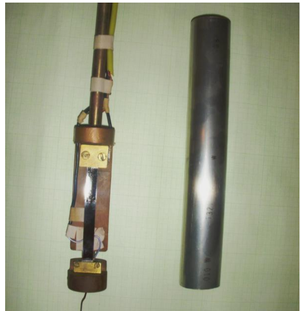
Fig. 3. View on holder and stainless steel cover.
