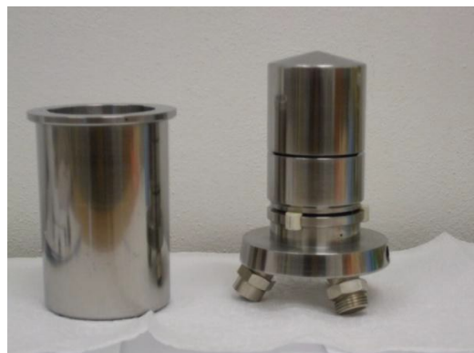
Fig.3. Container on measurement C_x and \tan \delta of liquid insulators [2].
