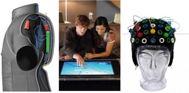
Figure 2. From left: I-Garment is developing full-bodied smart garments – to be worn by fire-fighters and the like – that monitor and transmit the location and vital signals of its wearer (such as body temperature and heartbeat).
