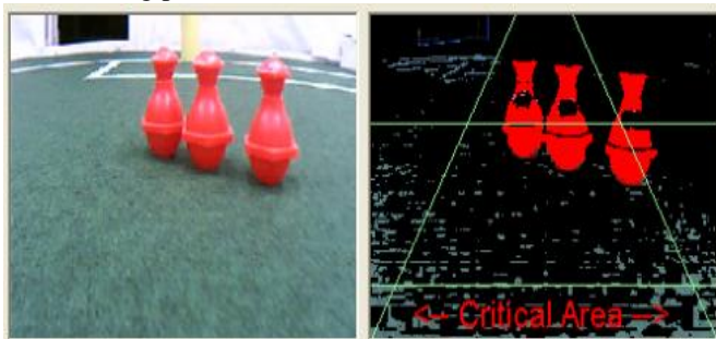
Fig. 2 Example of segmented image generated in the second phase of IP
