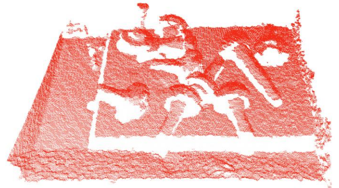
Fig. 2. Typical Kinect input data with point cloud data representation. Several particles may be seen in the image. Point cloud distances should correspond to distances in meters.
