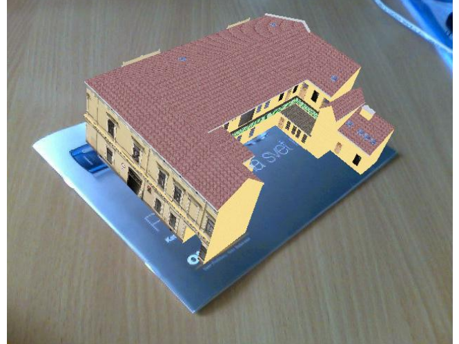
Fig. 5. Semi-markerless AR system. The virtual model is displayed in the real world.
