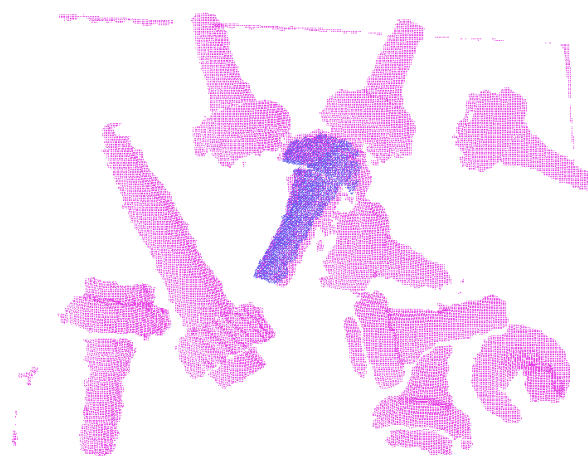
Fig. 6. Result of particle localization. The transformed model is shown in blue. The model particle and one of the scanned particles overlap, thus the result is satisfactory.
