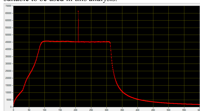
Fig. 4. Extreme erroneous value measured by the RPM sensor (x axis- time samples ; y axis - RPM)
