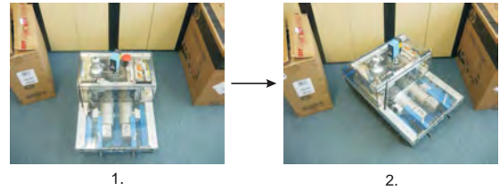
Fig. 8. The simplified space for comparison of the map, 1. vehicle position in the center of coordinates, 2. vehicle position after application error of the position
