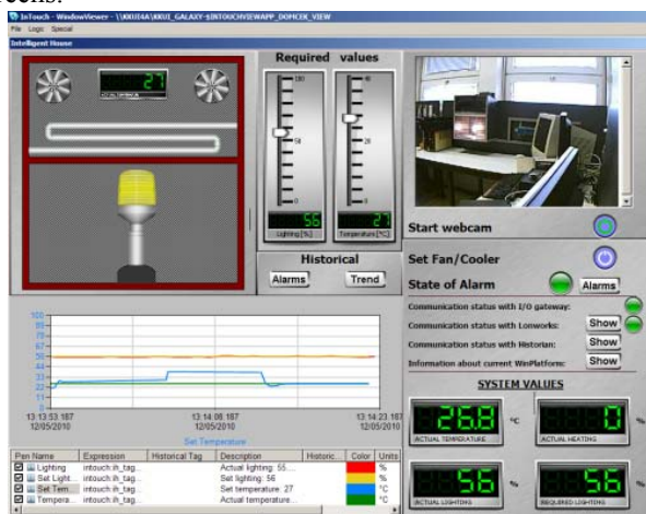
Fig. 4 Visualization application of controlled model Intelligent House created in ArcestrA IDE
