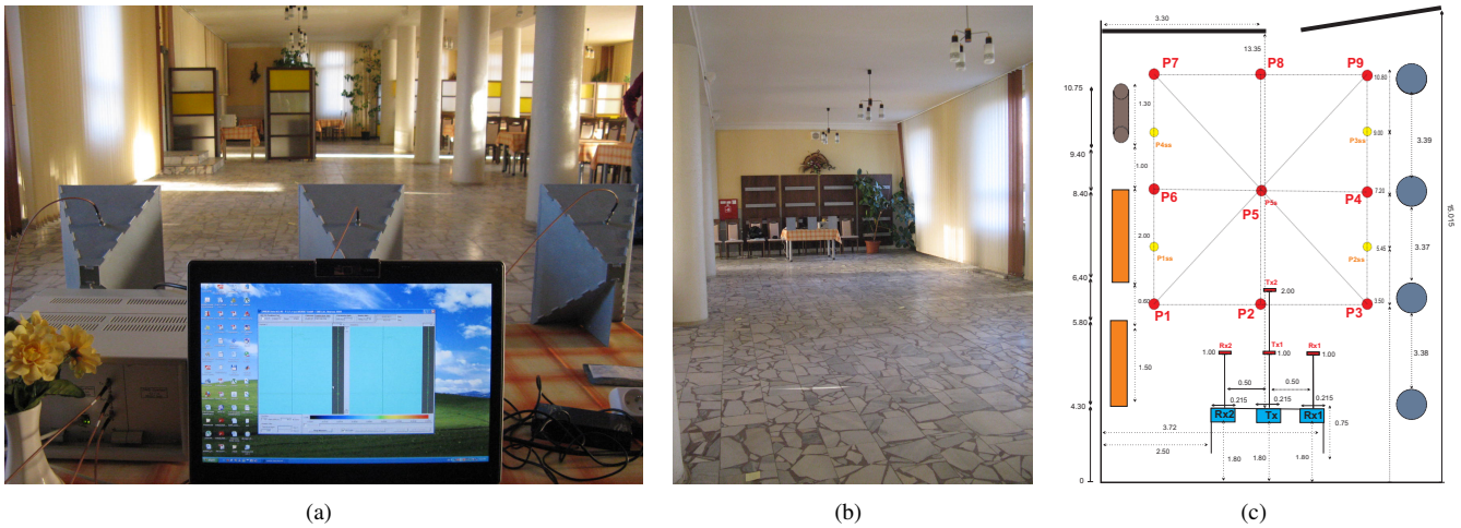
Fig. 1. The setup of UWB radar device in the school dining room for measurement of the shadowing effect, (a) view from behind of the radar device, (b) view from behind of the area of interest, (c) the scheme of the area with the reference points.
