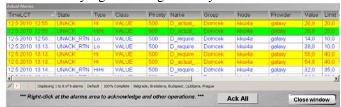
Fig. 5 Actual alarms window with the AlarmClient ArcestrA symbol
