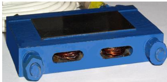
Fig. 1. Elastomagnetic sensors manufactured on KTEEM 120kN
