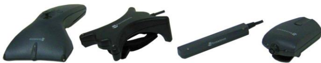
Fig. 7. MicroTrax devices (from left to right) – wand, hand tracker, head tracker, wireless transmitter
