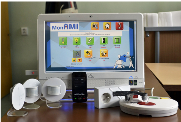
Fig. 6. Final solution with Asus touch screen, sensors and care phone unit
