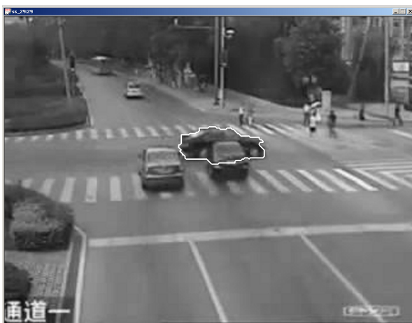
Fig. 4. : Segmentation by graph-cut based method. Segmented object is occluded by car.
