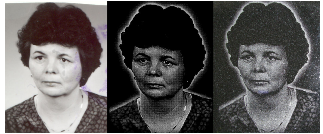
Fig. 6 Original grayscale photo (on the left), binary image (in the middle) and image engraved into black granite (on the right)
