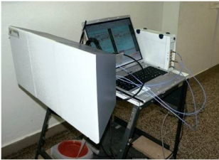
Fig. 1: M-sequence UWB radar system with horn antennas.
