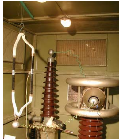
Fig. 1. Location of the test coil to measure partial charges
