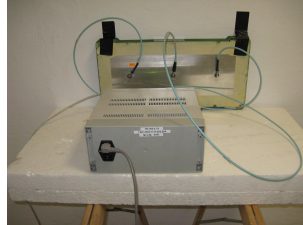
Fig. 2: M-sequence UWB radar system with spiral antennas.
