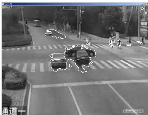
Fig. 3. : Segmentation by threshold based method where object contour detection fails
