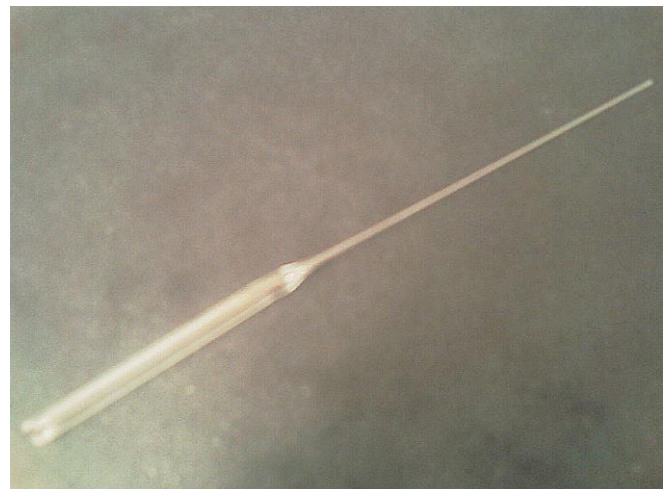
Fig. 3. Glass capillary. One of capillary which was hand made and used. On the picture we can see unevenness of the capillary, which produces defocusing of microscope view and moving sample out of field of microscope view.
