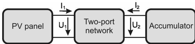
Fig. 3. Connection between a PV panel and an accumulator with general two-port network.
